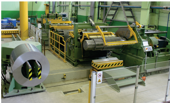
THE SLITTING AND CUT-TO LENGTH LINES FOR ELECTRICAL STEEL (GEORG COMPANY)
