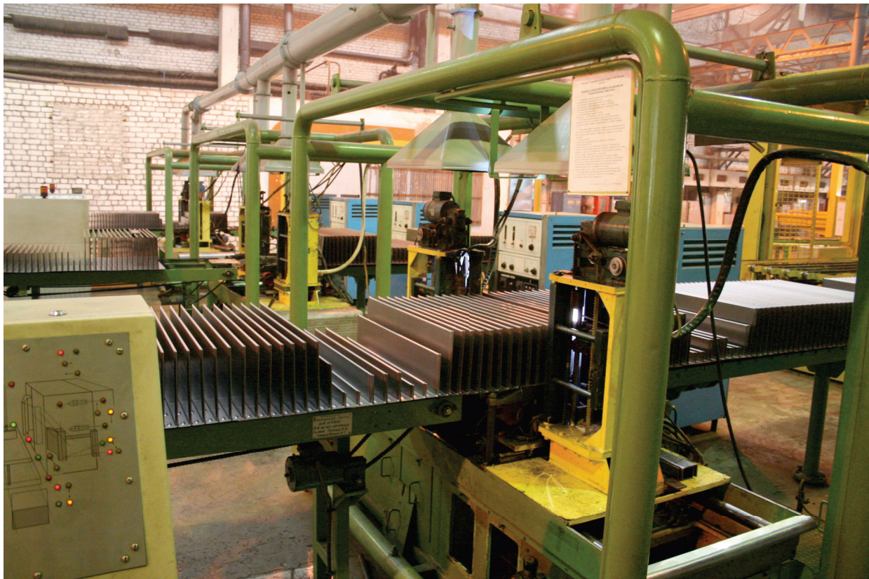
LINE FOR PLASMA WELDING OF CORRUGATED WALLS
