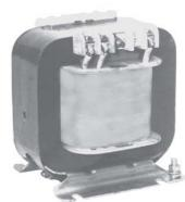
Transformers employ a strip-wound split-type magnetic core of cold-rolled electrical steel. Transformer coils are bobbin-type, made of copper wire with heat-resistant insulation. Assembled transformers are impregnated with wet-strong insulating varnish in a vacuum impregnator.
